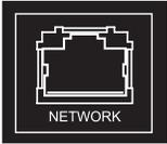
Configuring Anthem Room Correction, streaming or using IP control requires a network connection. To use a wired network connection, connect your SLM to a router using a 10/100 Ethernet cable.
