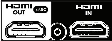
Insert HDMI cables gently, as the connector is more delicate than traditional ones. Damaged cables can damage jacks, and the warranty does not cover jack replacement. Therefore, replacing HDMI cables is recommended if there is any chance of damage with the existing cable.
